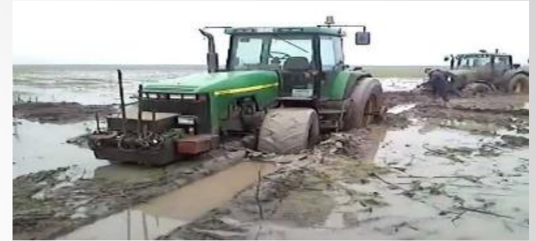
Tractor stuck in the mud due to high soil moisture content.
