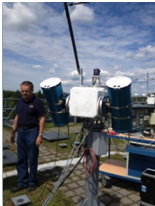
Figure 1. PSR#004 and PSR#006 installed on a sun-tracking device at MOL-RAO.
